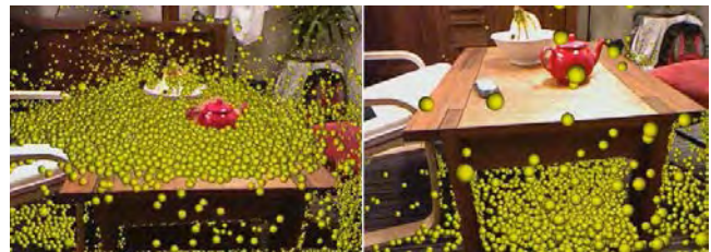
Figure 14: Thousands of particles interact live with surfaces as they are reconstructed. Notice how fine-grained occlusions are handled between the real and virtual. Simulation works on the TSDF volumetric representation, and runs on the GPU alongside tracking and mapping, all in real-time.
