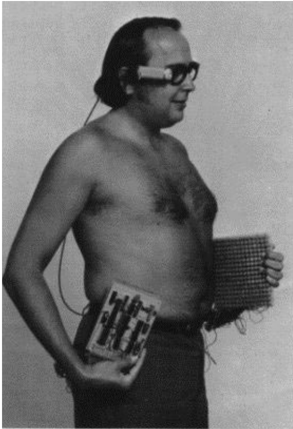
Figure 7. A blind subject with a “Tactile Visual Substitution system” (TVSS). A TV camera (mounted on spectacle frames) sends signals through electronic circuitry (displayed in right hand) to an array of small vibrators (left hand) which is strapped against the subject’s skin. The pattern of tactile stimulation corresponds roughly to a greatly enlarged visual image. (Photograph courtesy of P. Bach-y-Rita). From Morgan (1977).
