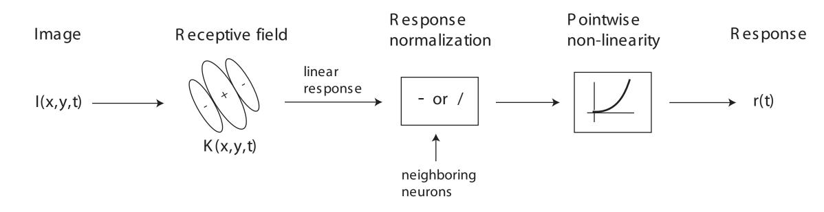
Here we consider a somewhat simpler version without the response normalization step. The neuron's response r is modeled by computing the convolution of the image I(x,y,t) with a space-time kernel K(x,y,t) and passing the result through a point-wise non-linearity, plus an offset:
