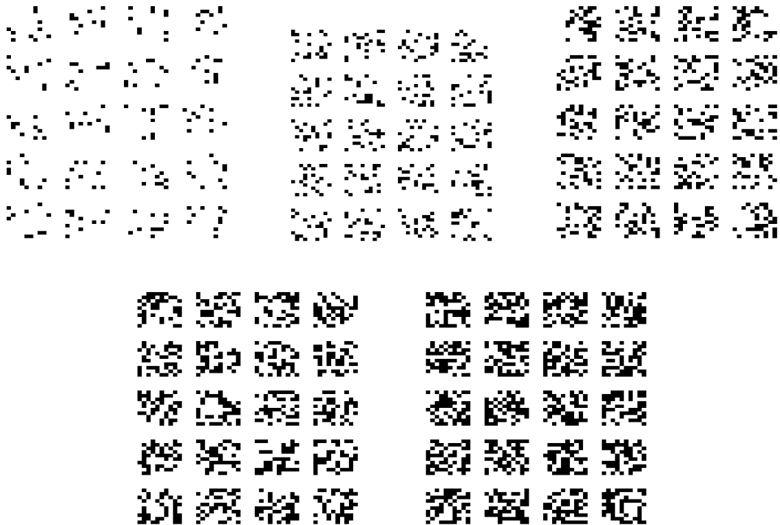
Figure 4: A sample set of sparse patterns used to explore the capacity of the network. Displayed left to right, the sparsities are at 10, 20, 30, 40, and 50 % of the image.
